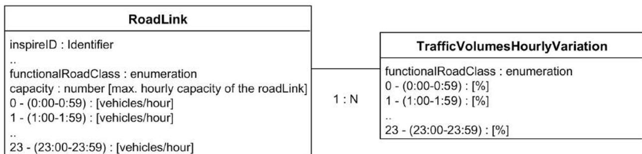
**Figure 5. Enrichment of transportation network data structure by hourly variation of traffic volume.**
